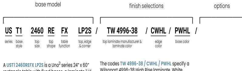
A **UST1 2460REFX LP2S** is a Uno<sup>2</sup> series 24" x 60" rectangle table with fixed bases, a laminate 1 1/4" thick top with a PVC edge and square corners.
