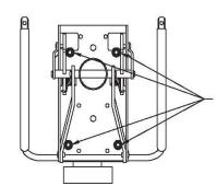
(4) OUTER HOLES OF TOP PLATE ARE PRE-DRILLED IN TOP FOR LOCATING
